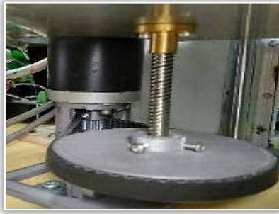
Figure 10: DC motor connected to a threaded rod via belt and pulley mechanism
