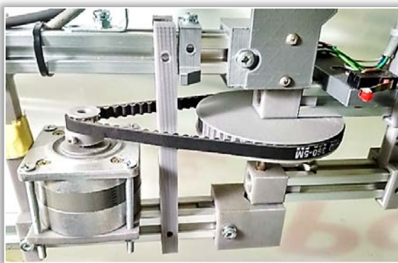
Figure 12: Pulley and motor assembly for elbow
