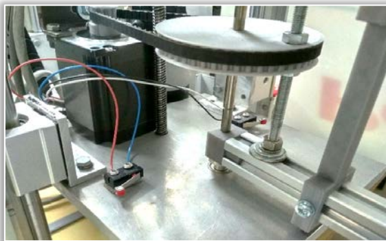
Figure 11: Pulley and motor assembly for shoulder
