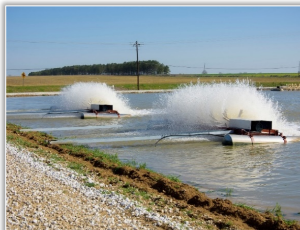
Figure 1. Pump sprayer aerator in operation
