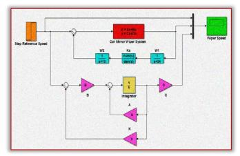
Figure 4. Simulink model of the vehicle windshield wiper system using H infinity Loop Shaping and Robust Pole Placement Controllers for tracking the step speed reference The wiper system performance for the proposed controllers using a step reference (step change from 0 to 6 m/s) of the wiper speed simulation is shown in Figure 5 below.
