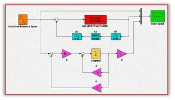
Figure 6. Simulink model of the vehicle windshield wiper system using H infinity loop shaping and robust pole placement controllers for tracking the sine speed reference The wiper system performance for the proposed controllers using a sine wave reference (wiper moving in the forward and reverse with 6 m/s) of the wiper speed simulation is shown in Figure 7 below.
