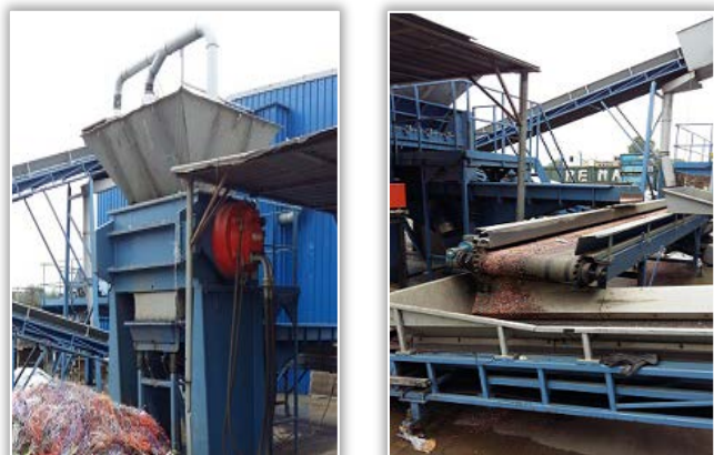
Figure 5. a) Super Chopper, b) Vibrating trough and conveyor belts
