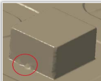
Figure 6. Irregularities on the triangulated cloud point
