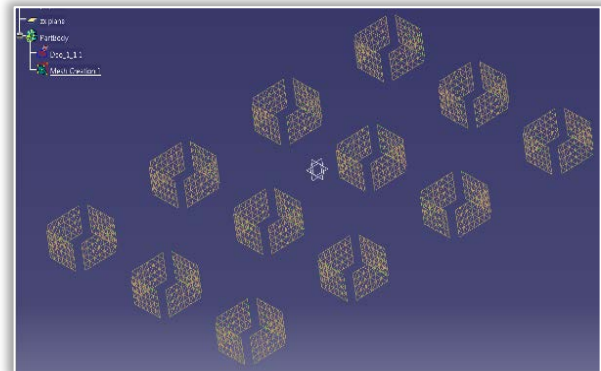
Figure 4. XYZ file imported to MeshLab and the triangulated point cloud in CATIA
