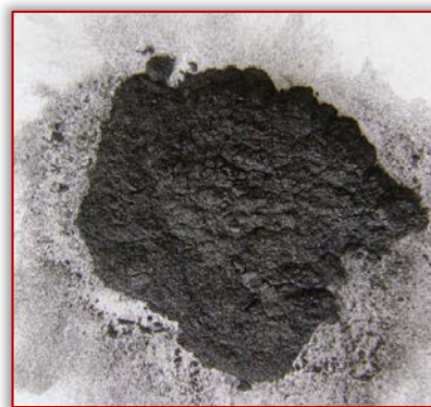
Figure 5. The powder separated after washing and filtration process
