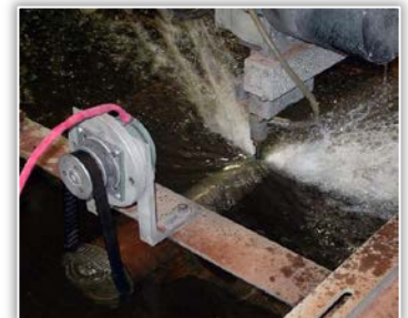
Figure 2. Delaboration of projectile by applying AWJ technology
