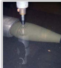
Figure 2. Delaboration of projectile by applying AWJ technology
