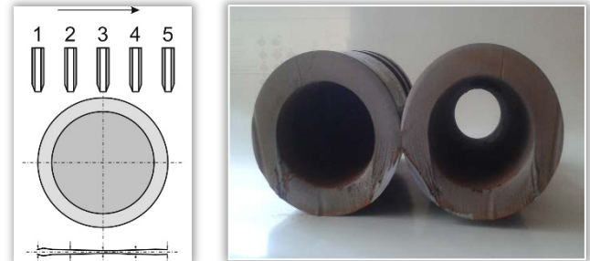
Figure 5 Display of the 100 mm caliber projectiles when cutting using AWJ
