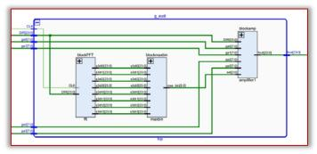
Figure 2: Schematic of the Algorithm Implementation. ADAU1761 codec of Zedboard was utilized to accept audio signal through line in channel. GPIO ~1 is the audio input and GPIO-O is the processed output. Figure 3 is the complete schematic including codec and algorithm.
