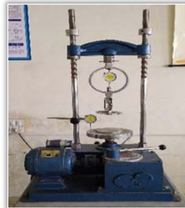
Figure 3. Determining the UCS
