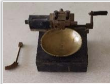
Figure 1. Determining the plasticity index
