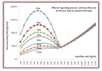
Figure 5. Two Phase Flow pressure drop in the HCE, this work
