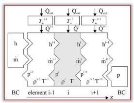
Figure 4. Axial discretization of fluid and pipe sections [20]
