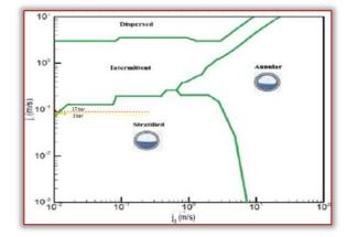
Figure 6. Surface velocities of two pressures 17bar and 3 bar in a DSG flow pattern map by Zarza [15]
