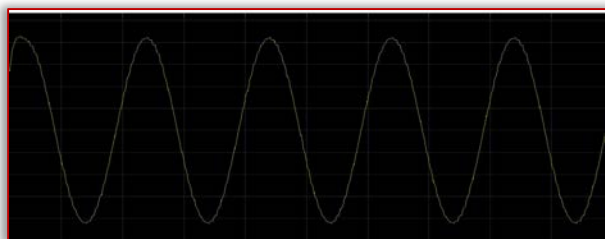
Figure 19. Inverter output after passing through Filter
