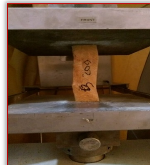
Figure 1: Failure mode of 200mm (Shear)
