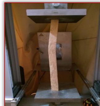
Figure 3: Failure mode of 200mm (Buckling)
