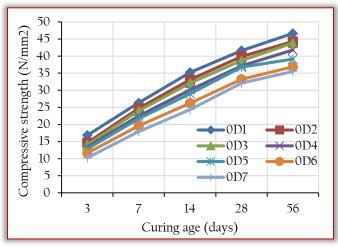
Figure 2. Relationship between the compressive strength and curing age of concrete specimens containing 0% sugar cane bagasse ash (SBA) and saw dust ash (SDA)
