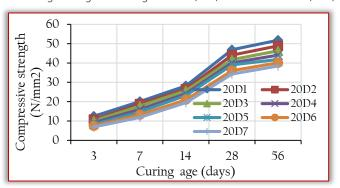
Figure 4. Relationship between the compressive strength and curing age of concrete specimens containing 20% sugar cane bagasse ash (SBA) and saw dust ash (SDA)
