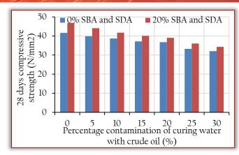
Figure 6. Relationship between the percentage contaminations of curing water with 28 days compressive strength of concrete specimens containing 0% and 20% sugar cane bagasse ash (SBA) and saw dust ash (SDA)
