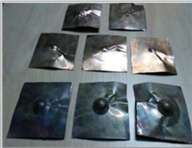
Figure 2. Erichsen cupping test – copper foil
