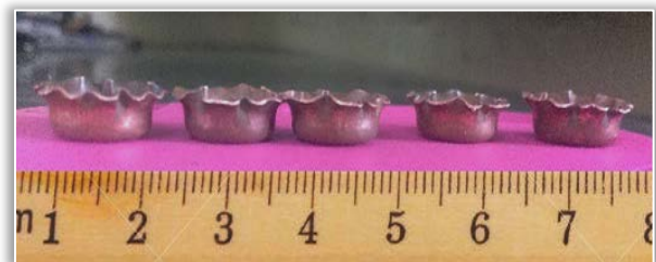
Figure 4. Cups formed with different initial thickness
