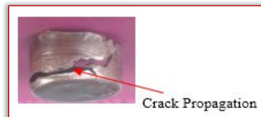
Figure 5. Failure by crack propagation
