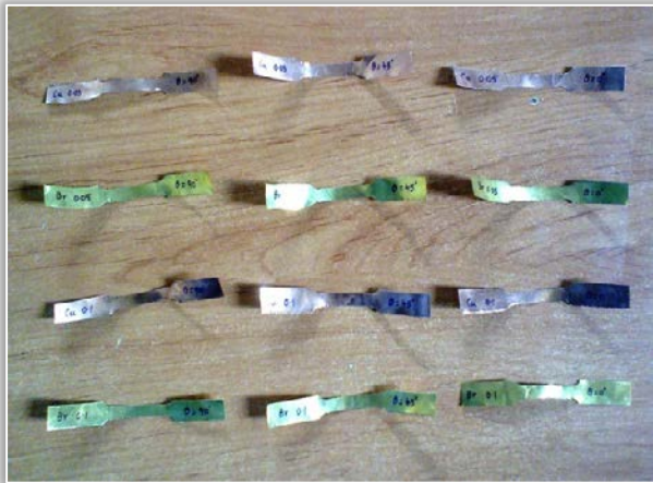
Figure 1. Micro tensile test – copper C1100 foil
