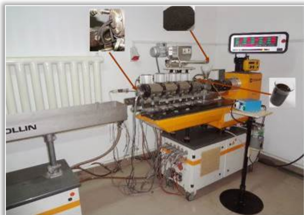
Figure 2 – Extrusion plant type „ZK 25“, production Collin
