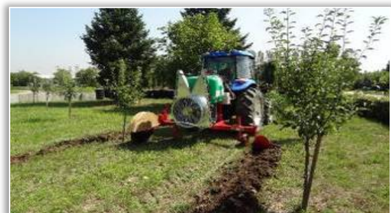
Figure 5 - Aspect during the determination of energetic indexes for the aggregate TD 80D New Holland tractor + ETR technical equipment during root cutting and soil processing works
