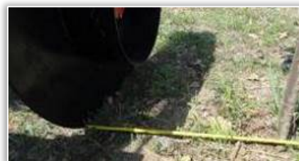
Figure 3 - Measuring the distance from the trunk to the root cutting disc
