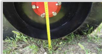
Figure 2 – Measuring root cutting depth
