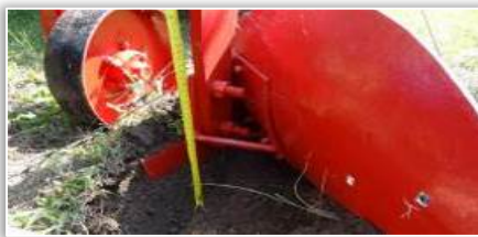
Figure 4 - Measuring soil working depth
