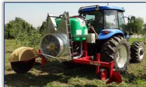
Figure 1 - Technical equipment for working the soil in the row of fruit trees along with root cutting to moderate shoots growth and precision foliar fertilization, ETR
