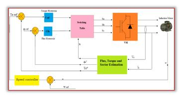
Figure 1. Basic DTC control scheme for IM.
