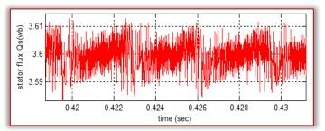
b) DTC-ANN with ANFIS speed regulator Figure 14 Zoom in the stator flux.
