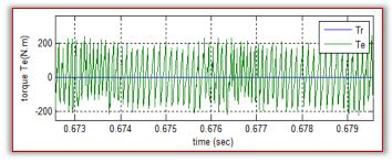
b) Neural DTC with ANFIS speed controller Figure 13 Zoom in the torque.
