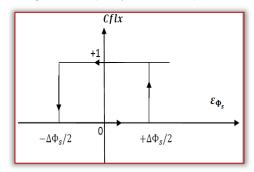
Figure 4. Flux hysteresis comparator.
