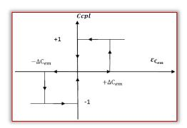
Figure 3. Torque hysteresis comparator
