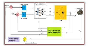
Figure 5. DTC-ANN with ANFIS speed controller.
