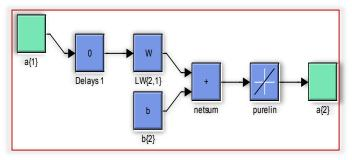
Figure 8. Structure of layer 2
