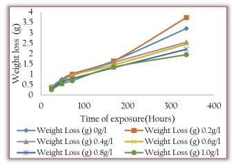
Figure 4: Variation of weight loss with time for the corrosion of AISI 1007 Steel in 2M HCl The variation of weight loss against time of exposure for corrosion of AISI 1007 Steel in 2M HCl containing various
