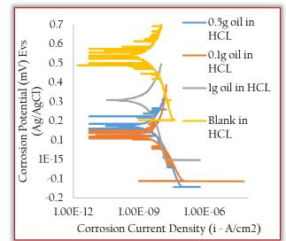
Figure 8: Corrosion Potential against Corrosion Current Density (Cucumber Seed Oil)
