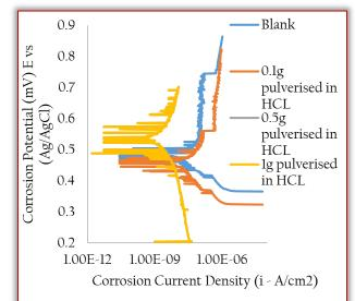
Figure 7: Corrosion Potential against Corrosion Current Density (Pulverised Peel)
