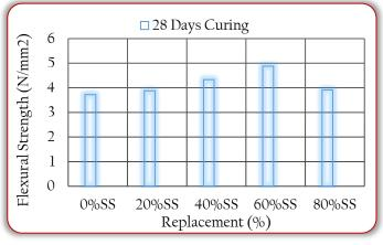
Figure 14: Effect on Flexural Strength of Steel Slag (Thangaselvi 2015)
