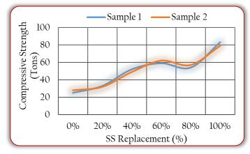
Figure 1: Effect of Steel Slag on the Compressive Strength at 28 day curing (Gokul et al., 2012)
