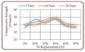
Figure 3: Steel Slag Compressive Strength (Raza et al., 2014) The research conducted by Thangaselvi (2015) as seen in Figure 4 shows that the compressive strength of concrete increases up to 60% (with an increment of 9.70%) replacement of coarse aggregate with steel slag but the strength decrease at 80% replacement. This is guite in agreement with the previous study conducted by Gokul et al. (2012).
