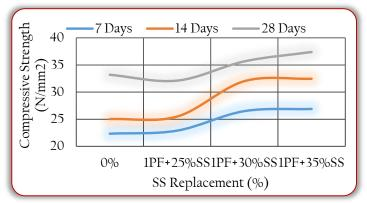
Figure 2: Compressive Strength of Concrete Grade 30 (Kumar and Kumar, 2016)
