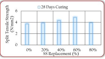
Figure 9: Split Tensile Strength of Steel Slag Concrete (Thangaselvi, 2015)
