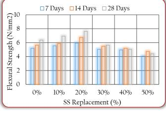
Figure 13: Flexural Strength of Steel Slag Concrete (Raza et al., 2014)
