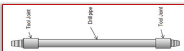
Figure 2. Drill pipe in general
