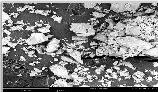
Figure 8a. SEM micrograph of 40 wt. % SP reinforced carbon composite
