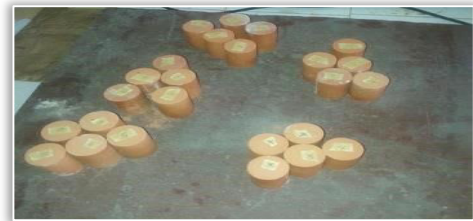
Figure 3. Compacted silica reinforced carbon matrix composites (a) Green compacts (b) Sintered samples
