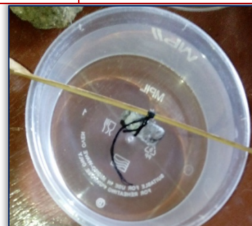
Figure 4: Picture of corrosion setup
