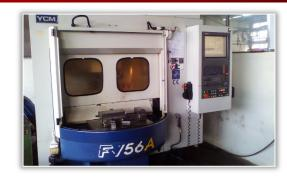
Figure 7. CNC Milling machine [8]
