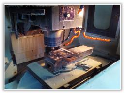
Figure 11. Production of tool part with CNC Milling machine [8] B. Mechanical part (complex geometry)
