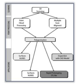
Figure 2. Reverse Engineering – the generic process [1] Reverse Engineering strategy must consider the following: Reason for Reverse Engineering of a part
