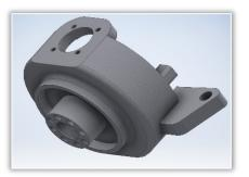
Figure 13. CAD model of the mechanical part After we have made the measurement of the existing work piece and creating the 3D model through the software (Figure 13), the next step was the manufacturing on the milling machine (figure 14).
