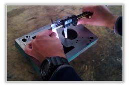
Figure 9. Measurement of tool part [8] After we have made the measurements of the existing work piece (Figure 9) and created a 3D model through the software
