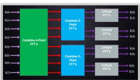
Figure 8. Radix-2 mechanism of FFT
