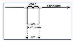
Figure 3. Schematic of current sensor's connection
