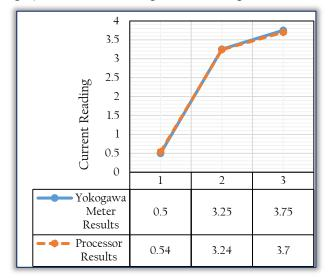
Figure 12. Current comparison between microcontroller and meter reading
