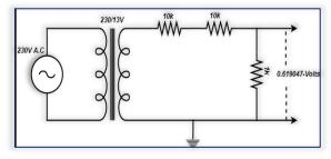
Figure 1. Schematic of voltage sensor's connection
