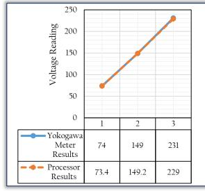
Figure 10. Voltage comparison between microcontroller and meter reading
