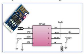
Figure 5. Schematic of ESP8266 Wi-Fi module
