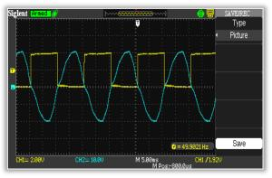
Figure 4. Output of zero crossing detector
