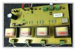
Figure 6. Voltage sensor's hardware PCB
