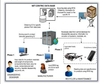
Figure 1. Flowchart of the proposed model for nondestructive disassembly using augmented reality and RFID technology
