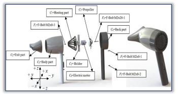
Figure 2. Exploded view and assembly of hair-dryer The electric motor as valuable component of interest for reuse is aim for the disassembly process. The optimal disassembly sequences in according with methodology presented in the paper [11] are:
