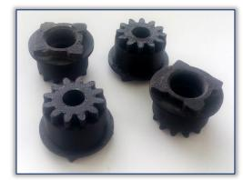
Figure 7. Small batches of gears made in the integrated process of additive manufacturing technology and vacuum casting **CONCLUSIONS**
