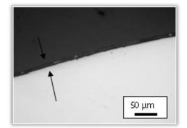
Figure 2. Galvanized (zinc-coating) layer of the chains (thickness 12 mm)
