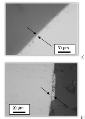
Figure 1. Galvanized (zinc-coating) layer of the chains (thickness 9 mm)
