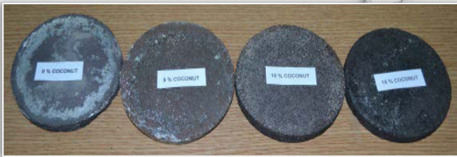
Figure 1. Specimen of composite material using for mechanical tests
