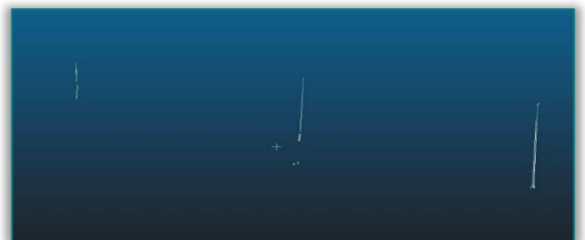
Figure 26. Extracted points representing poles of street lamps
