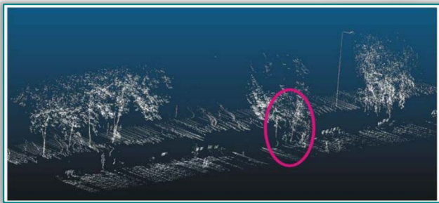
Figure 13. Example of the point cloud after extraction of road surface and building facades
