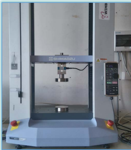
Figure 7. Testing machine with compressive module
