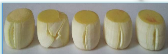
Figure 8. Samples for compressive testing: a) ABS, b) ABSplus, c) PLA
