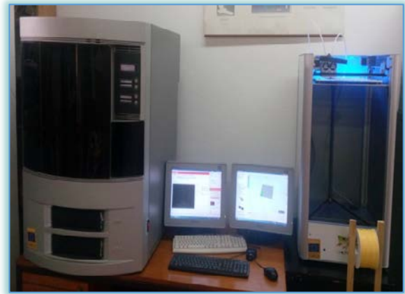
Figure 2. 3D printers: Dimension Elite (left) and LeapFrog Creatr XL (right)
