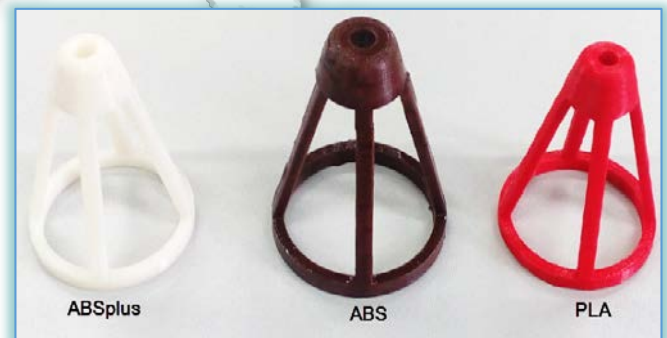
Figure 6. The holders produced using additive manufacturing technology
