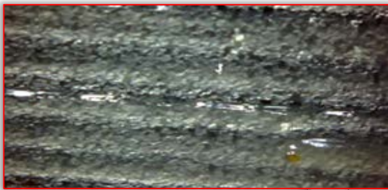
Figure 15. The sample after laser cleaning lubricant Berutox M 21 KN, mag.50x
