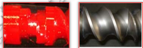
Figure 6. Extrusion screws before and after cleaning operation [7]
