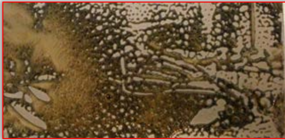
Figure 14. The sample after laser cleaning Berutox M 21 KN, mag.50x
