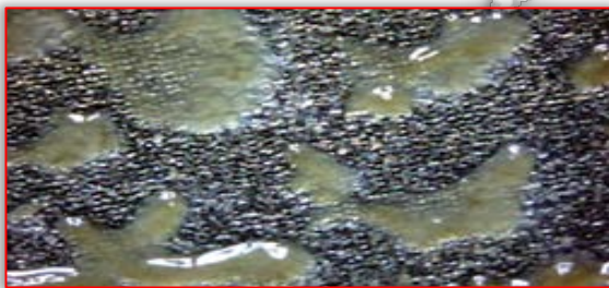
Figure 16. Detail of degreasing of lubricant Berutox M 21 KN, mag.50x
