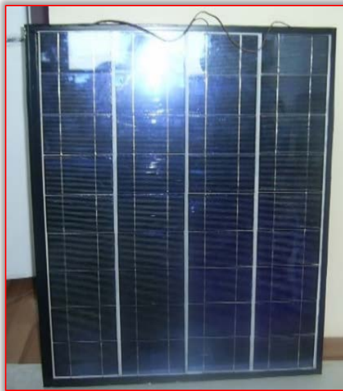
Figure 3. The first module – the photovoltaic panel [4-6] The first solar module consists of a handmade photovoltaic panel made from 36 solar cells that produces 65W and 3.6 A. [4-6]
