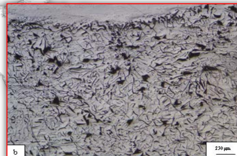
Figure 3. Microstructure after welding of cylinder head in the combustion chamber - a) and the base material - b)
