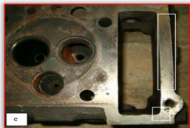
Figure 1. Cast iron cylinder head of a car Opel Omega 2.3 TD with the place of the samples
