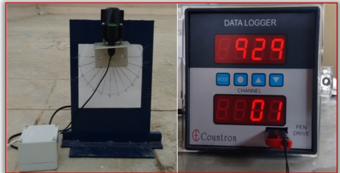
Figure 1. Pyranometer with data logger
