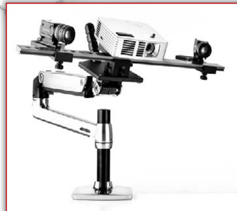
Figure 13. David SLS-3-STEREO structured light scanner
