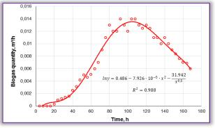
Fig. 2 –Variation of biogas production at 25°C
