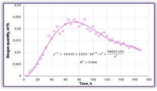
Fig. 4 - Variation of biogas production at 45°C the [2.] Experimental data, obtained from fermentation of a mixture of pig and cattle manure at different temperatures, in the pilot plant RE-biomass with continuous hydraulic stirred cylindrical digester, respectively 25°C, [3.] 35°C and 45°C, shows an increasing variation up to a certain moment in the process of fermentation, respectively a decreasing variation [4.] in the second part of the test that lasted for approximately 170 hours.
