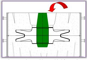
Figure 6. The mould assembled for casting
