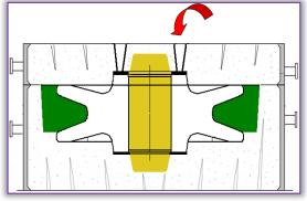
Figure 11. The mould assembled for casting
