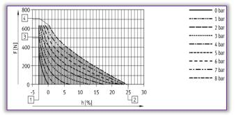
Figure 5. DMSP-10 muscle's force-contraction (relative displacement) diagram [21]
