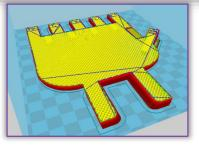
Figure 4. Hand in the 3D printer's slicing program Figure 3 and Figure 4 show the slicing program of the 3D printer. The parts in red represent the outer layer of the body, which the printer builds at a slow speed. The green and yellow parts refer to the filling of the body where the head works at a higher speed. Blue shows the lines where the head is inactive.
