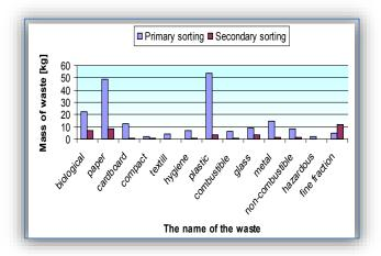
Diagram 2. Composition of remaining waste on the upper and middle sieve examination results
