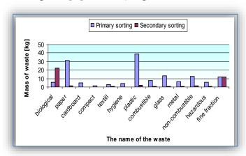
Diagram 1. Composition of remaining waste on the upper and middle sieve examination results
