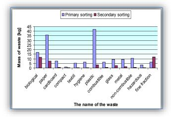
Diagram 3. Composition of remaining waste on the upper and middle sieve examination results
