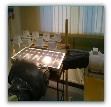
Figure 2. The illuminated PV module and the cooling system
