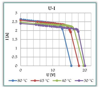
Figure 4. U-I characteristics in different temperatures
