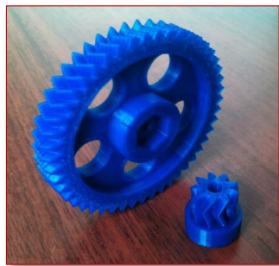
Figure 3. Self-replicating 3D printed gears
