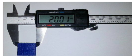
Figure 5. Self-replicating 3D printed – 20mm cube
