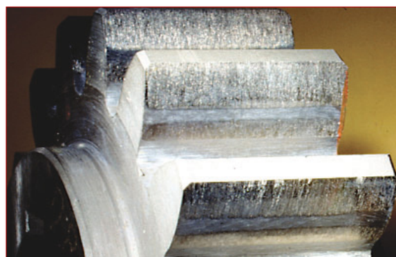
Figure 7. Gear scuffing failures [12]
