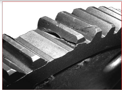
Figure 10. Breakage of more gearteeth [15]
