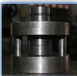
Figure 2. Micro Extrusion Die Assembly Table 1. Micro Extrusion Machine: Specifications
