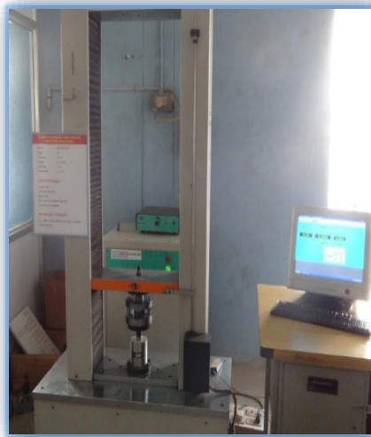
Figure 1. Micro Extrusion Experimental Set Up
