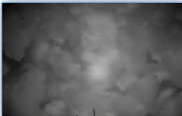
Figure 3(a): Optical Micrograph of the particles of silica gel at magnifications of 200X viewed using metallurgical microscope (AP2000 MTI). The micrographs showed that the particle sizes are on a micro particle scale of about 1.5 \mu\text{m} . The shape of the particle was found to be uniform and agglomerated.
