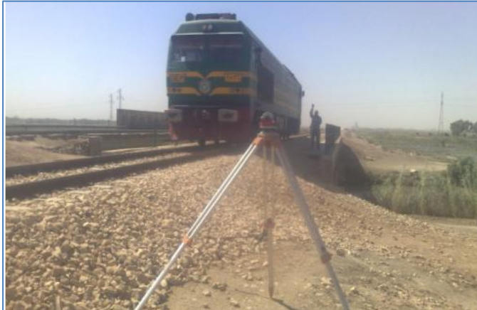
Figure 13. Method used for measuring deflections under dynamic live loading
