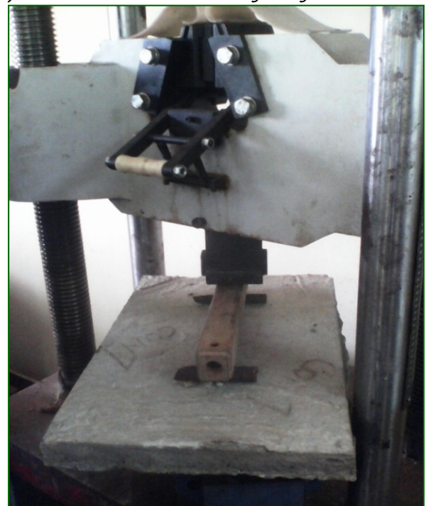
Figure 3: Slab specimen undergoing 3 points loading
