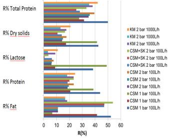
Figure 3: The retention values (R) of the different components were measured in 0.2 µm cut off value tubular membrane with (CSM+SK) and without static stirrer (KM-capillary membrane, CSM – tubular membrane)
