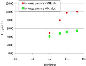
Figure 5: The changes of whey flux (J) as a function of trasnmembrane pressure at vibrated (54 Hz) and non vibrated methods
