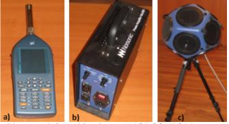
Figure 4 a) Sound level meter NORSONIC Nor 140. b) Noise generator Nor 280, c) Omnidirectional sound source NORSONIC 270 6. DETERMINATION OF THE SOUND INSOLUTION INDEX R'W AND INSTANCE A
