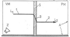
Figure 1. The principle of definition airborne sound insulation of the building construction Figure description:  $L_1$  – medium level of the sound pressure in volume room [dB],  $L_2$  – medium level of the sound pressure in receiving room [dB], 3 - decrease in the level of the sound pressure influence of sound insulation of the building structure.
