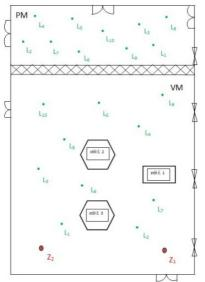
Figure 3. Positions of the microphones location in the receiving and volume room
