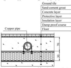
*Figure 2. Arrangement of floor heating coil pipe c) Natural Ventilation Enhance*
