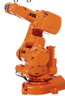
Figure 2. Industrial robot ABB IRB 140
